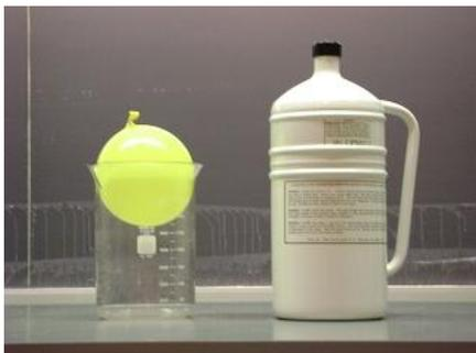
To demonstrate Charles' Law, liquid nitrogen is poured over a balloon filled with air.
